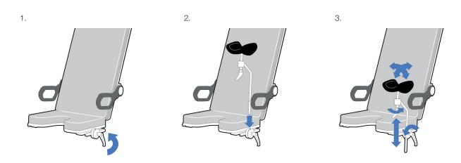
The leg rests include a block ring that prevents the leg rests from being lowered too far. The block ring must always be mounted onto the leg rest, if this is not used accordingly usage of the leg rests can result in patient or user injury.
